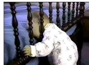
Trapped in Footboard
